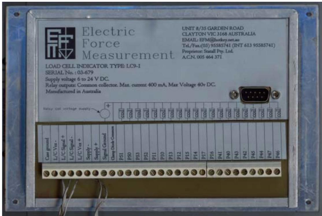
Power supply 8 to 24 volts DC or 6 to 18 volts AC
